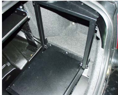
Position trunk side mount and determine where to notch vehicle trim in order to function properly
